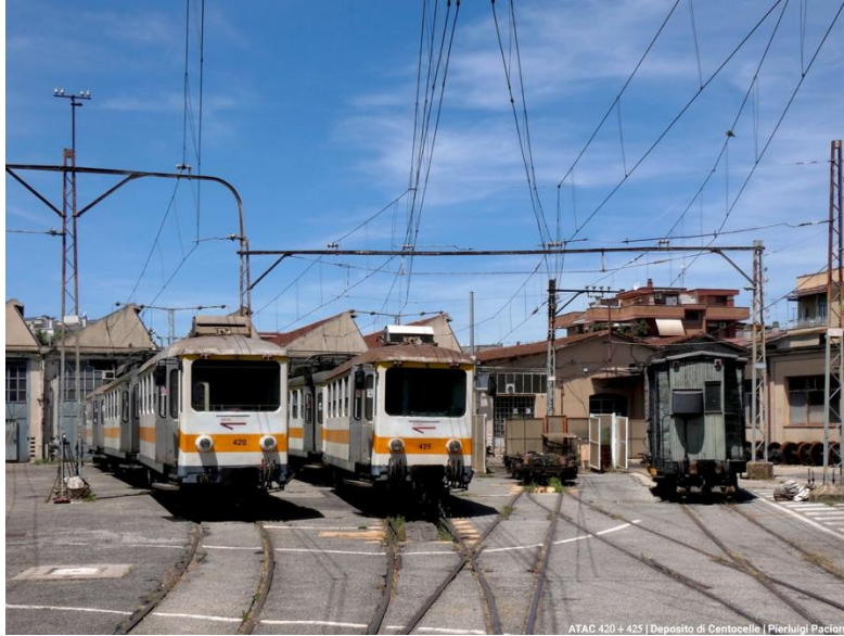
The internal yard of Centocelle depot today, still preserving the original poles and overhead line (photo taken by P. Paciorni, 2026).
